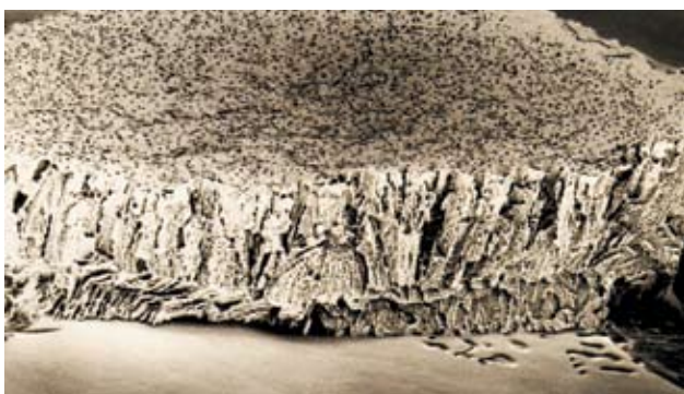
Figure 1: Cross-section of a lyophilized ODT showing the highly porous structure.
